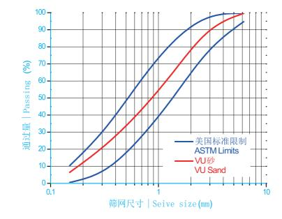
decreased, complying with the US standard ASTM C33, the Chinese standard JGJ52 (grading zone II) and the Indian standard IS 383 (grading zone II).
